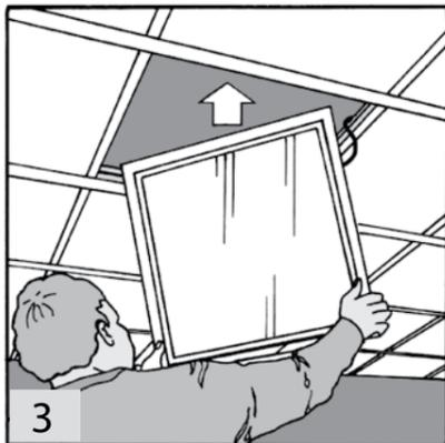
The light panel is being lifted through the hole in the ceiling system.
