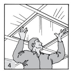
The light panel is lowered, and rests on the frames of the ceiling system. Make sure it is securely installed.
