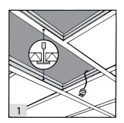
Winsta cables or cables mounted with Winsta connectors should be installed over the ceiling by an authorized electrician in the required length.
