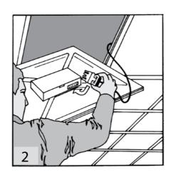
The Winsta cable is to be connected to the light panel. Due to the design of the Winsta connector, it can only be mounted in the correct polarization.
