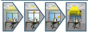
The lamp lights on 100% illumination or dims to maintain the preset illumination level against ambient light.
