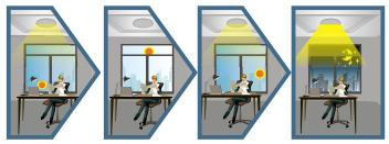
The lamp lights on 100% illumination or dims to maintain the preset illumination level against ambient light.
